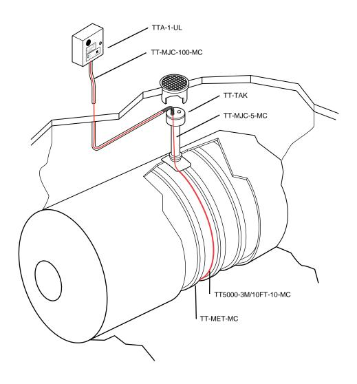
Typical bill of materials: Single-channel underground fuel tank sensor located 100 feet from the alarm module
