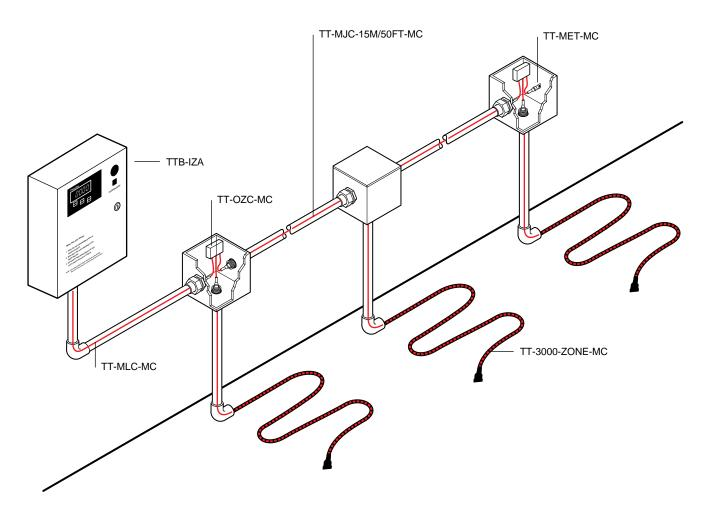
Typical bill of materials: Three-zone sump (monitoring watery waste sumps on 50-foot centers with the panel located 10 feet from the first junction box)
