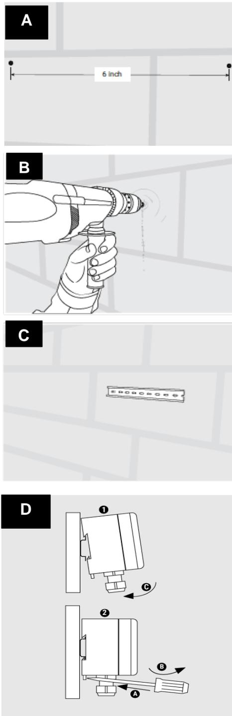
**Figure 2.1 – Mounting procedures for the 460 controller**
