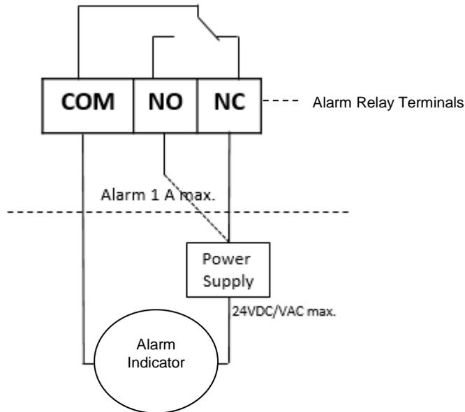
**Figure 2.5 – Alarm Wiring**
