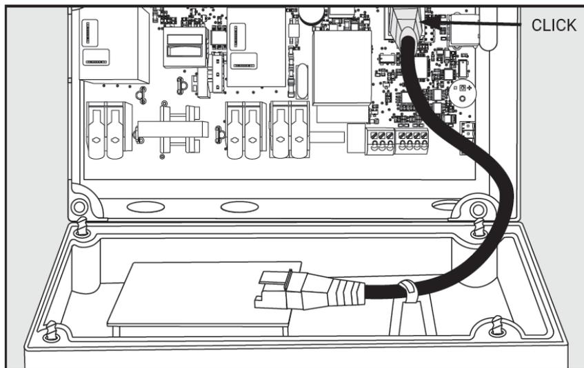
**Figure 2.6 – Connect the touchscreen cable to the controller.**
