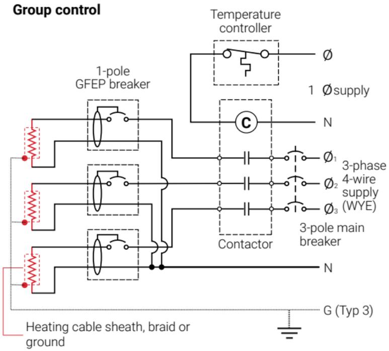
**Figure 5: Typical controller wiring—multiple circuits**
