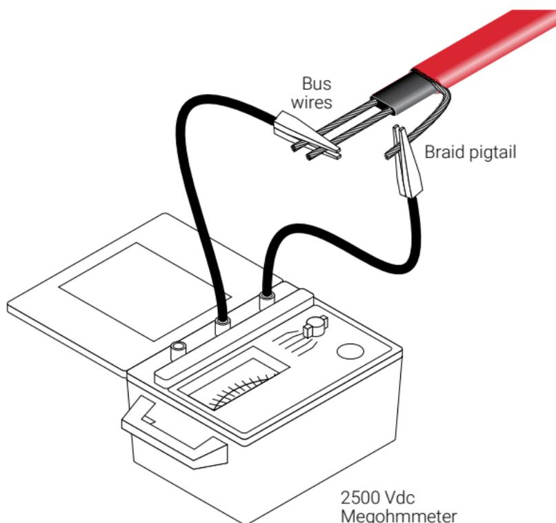
**Figure 7: Insulation resistance test**
