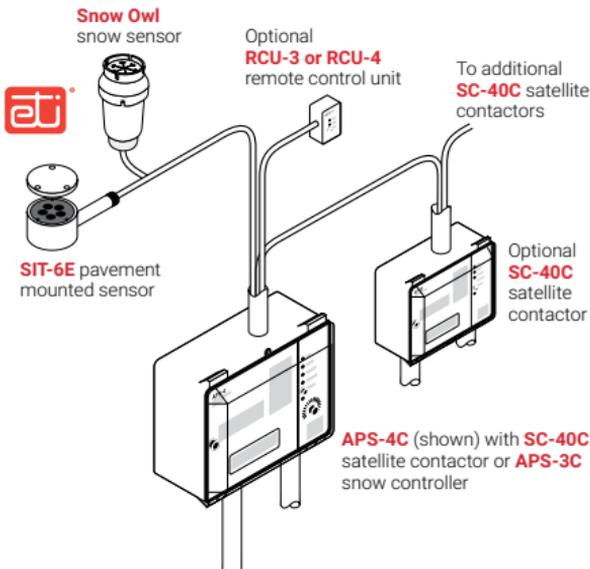
**Figure 4: Automatic snow melting control system**
