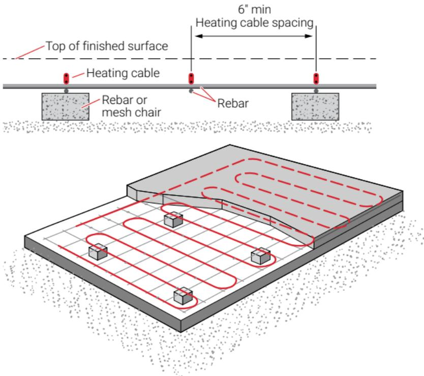
**Figure 4: ElectroMelt installed on rebar**
