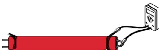
**Figure 8: Capacitance test**
