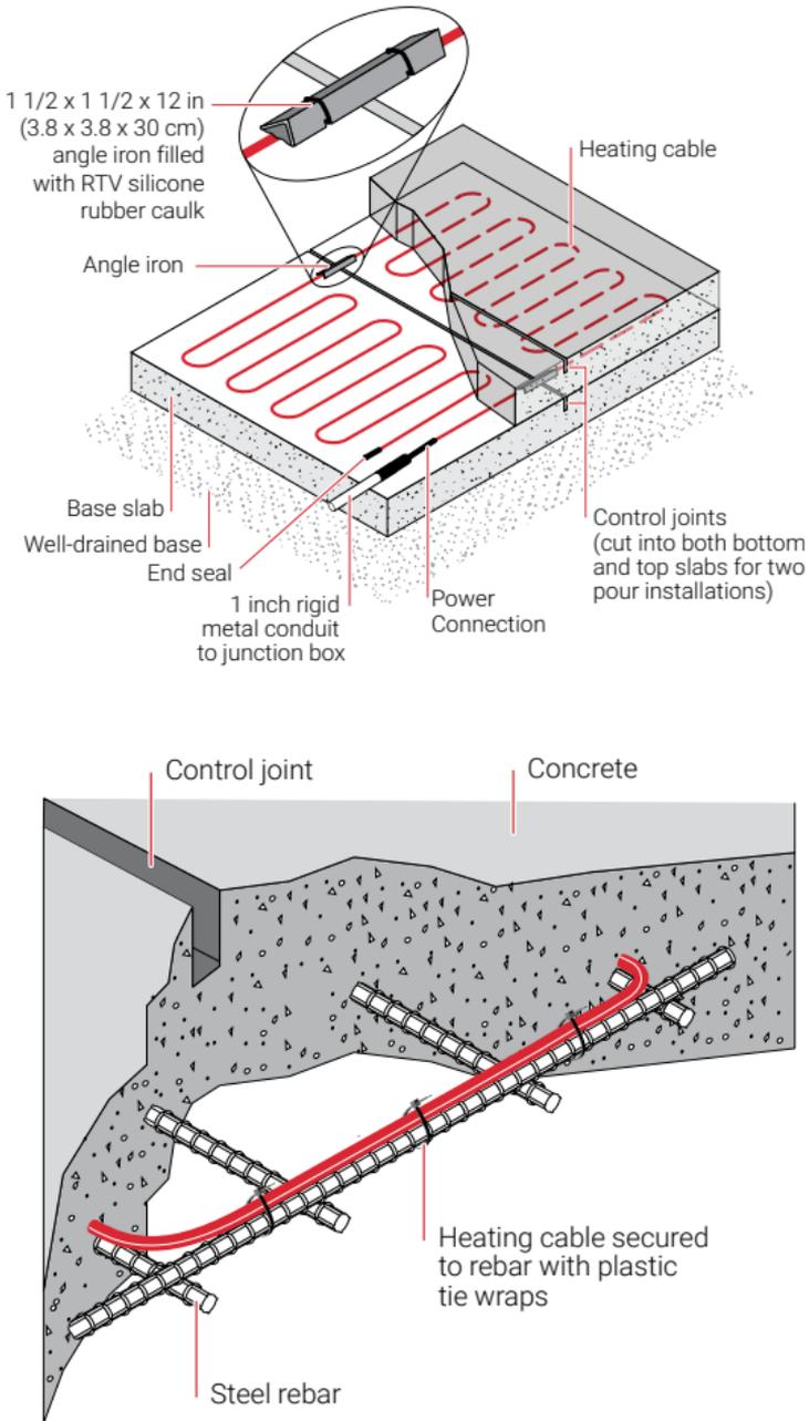
**Figure 2: Control joint**
