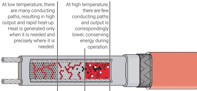
At low temperature, there are many conducting paths, resulting in high output and rapid heat-up. Heat is generated only when it is needed and precisely where it is needed.
