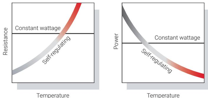
**Fig. 2 Self-regulating heating cable technology**
