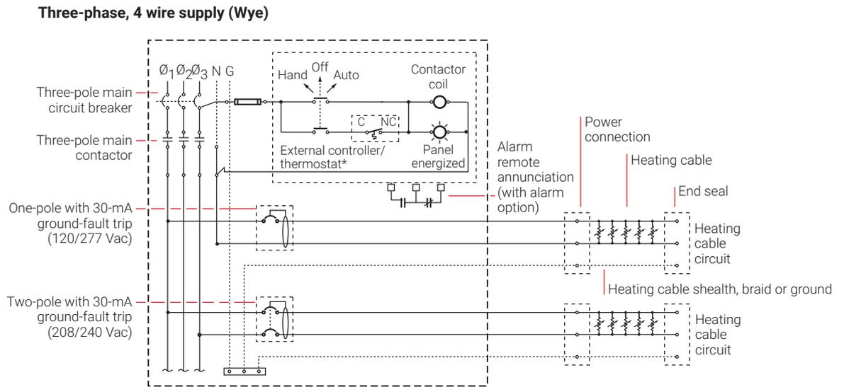
**Fig. 17 HTPG power schematic**
