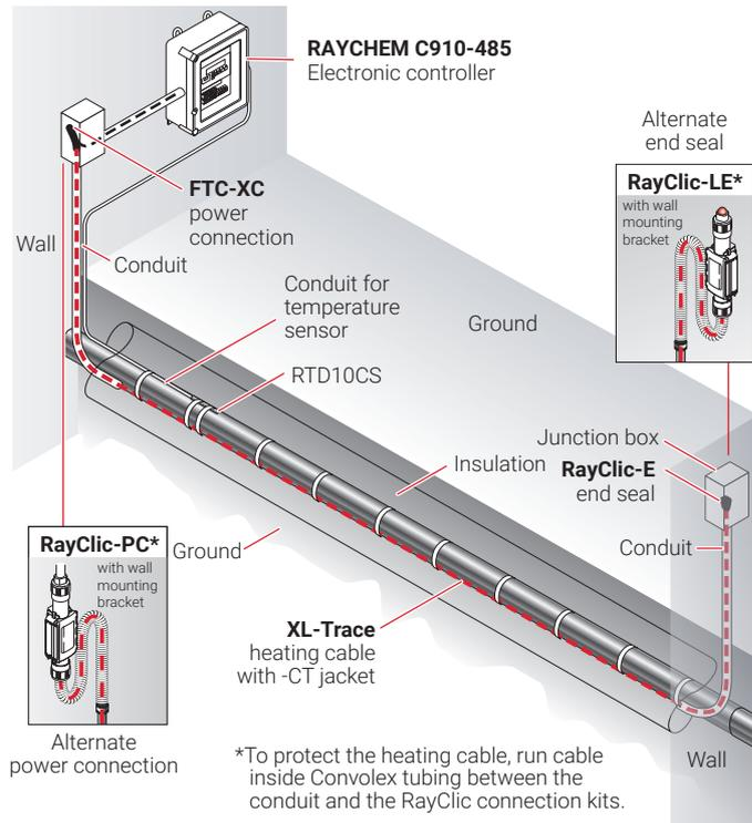
**Fig. 8 Typical buried grease waste line**
