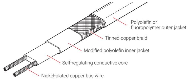
**Fig. 1 XL-Trace heating cable construction**
