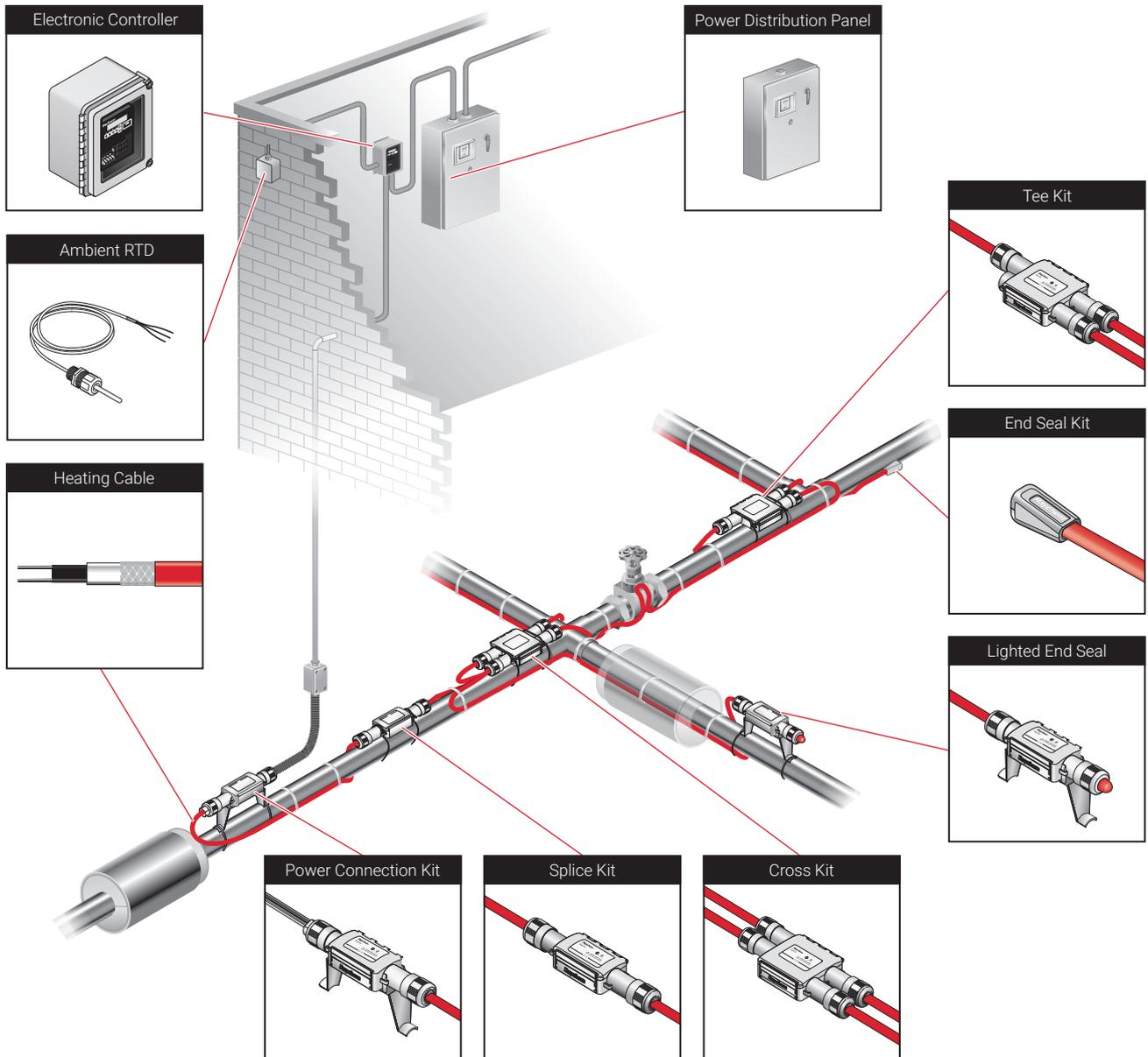
Fig. 3 Typical XL-Trace pipe freeze protection system
