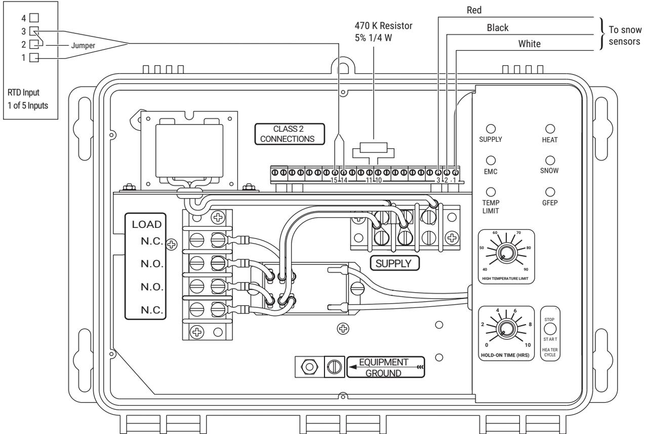
Fig. 5.7 Connecting the APS-3C
