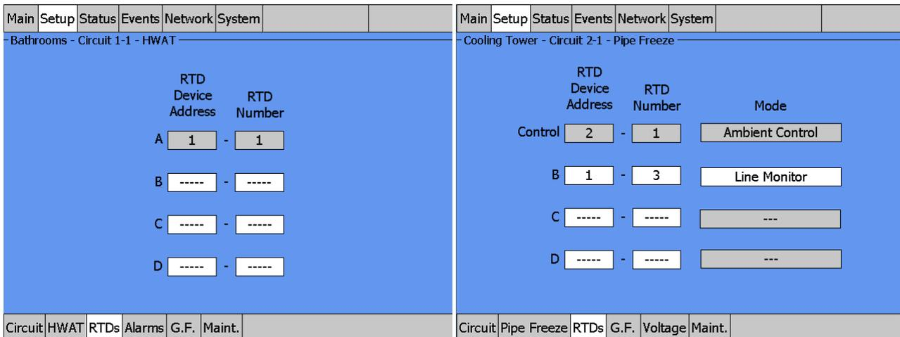
Fig. 3.26 Setup|RTDs window (Pipe Freeze Ambient Control)
