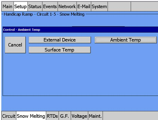
Fig. 3.102 Snow Melting - Ambient Temperature Control
