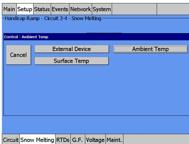
Fig. 3.97 Setup Snow Melting External Device Control window
