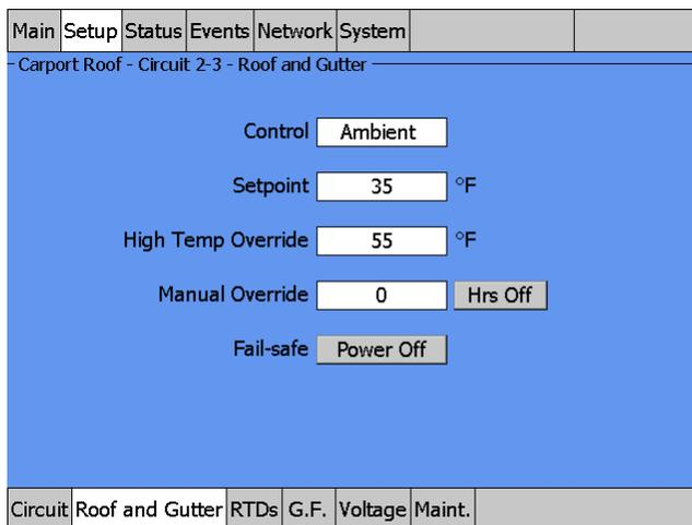
Fig. 3.79 Setup|Roof & Gutter - Ambient Temp Control Window
