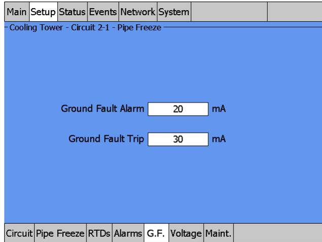
Fig. 3.42 Setup|G.F. window (Pipe Freeze PASC Control)
