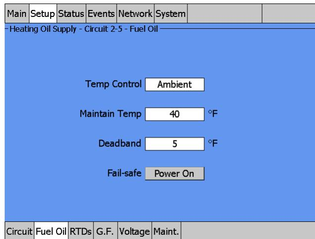
Fig. 3.46 Setup|Fuel Oil Ambient Control window
