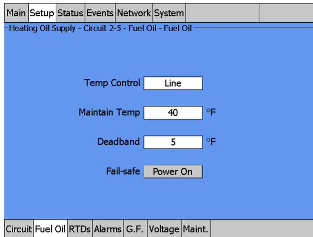
Fig. 3.53 Setup|Fuel Oil Line Control window
