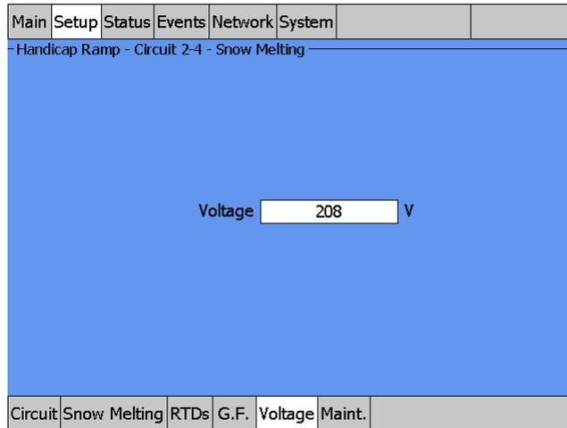
Fig. 3.94 Setup|Voltage Window (Roof & Gutter - Surface Temp Control)
