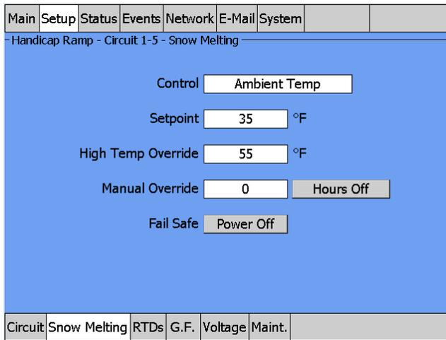
Fig. 3.103 Setup Snow Melting - Ambient Temp Control Window
