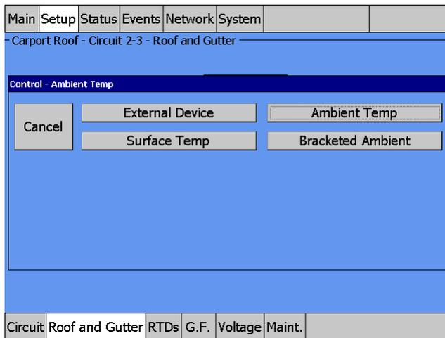
Fig. 3.78 Roof & Gutter - Ambient Temperature Control Window
