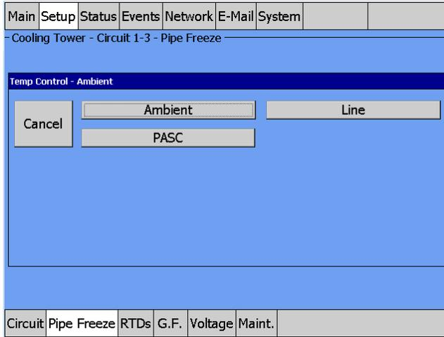
Fig. 3.24 Pipe Freeze Temperature Ambient Control window
