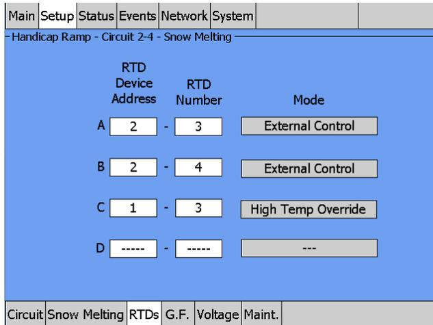
Fig. 2.17 External device RTD window
