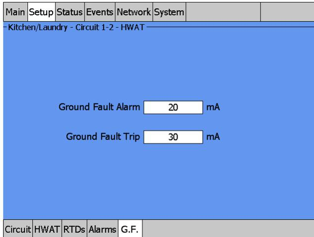
Fig. 3.11 Setup|G.F. window (HWAT)
