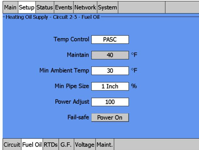
Fig. 3.60 Setup|Fuel Oil PASC Control window
