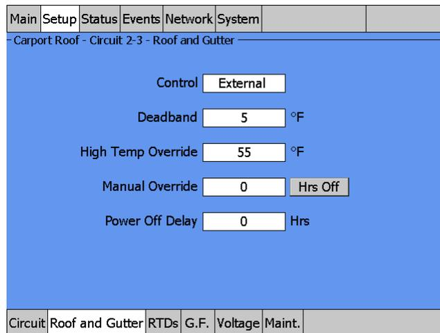
Fig. 3.73 Setup|Roof and Gutter External Device Control window
