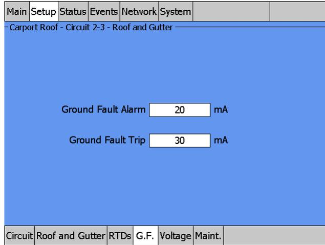
Fig. 3.75 Setup|G.F. Window (Roof & Gutter External Device)
