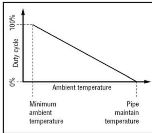
Fig. 5.1 Proportional Ambient Sensing Control (PASC)
