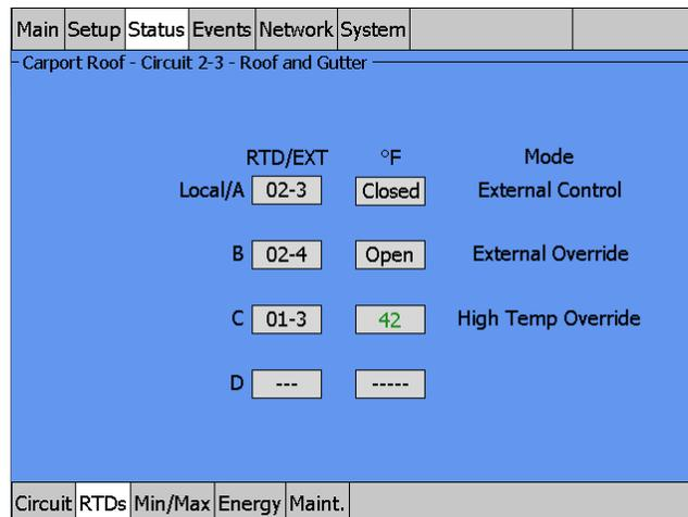
Fig. 2.27 Status|RTDs window - external device
