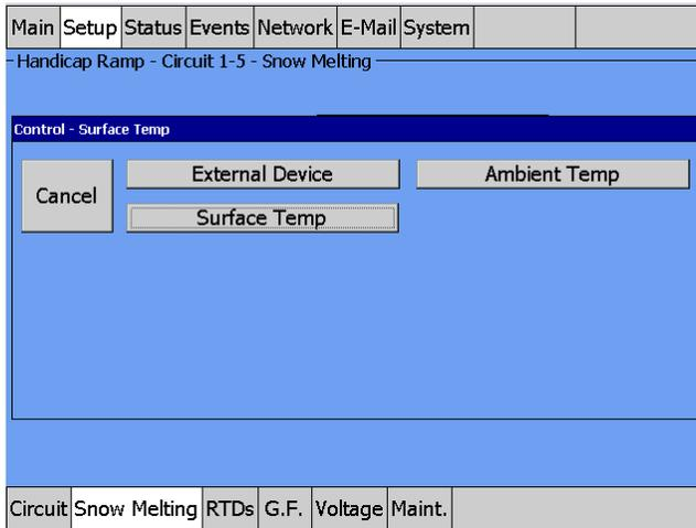
Fig. 3.108 Roof & Gutter Surface Temperature Control Window
