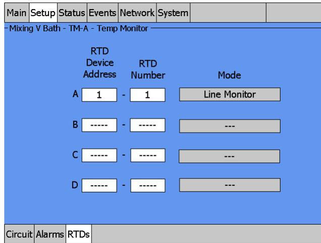
Fig. 4.4 Temperature Monitor - Assigning RTDs
