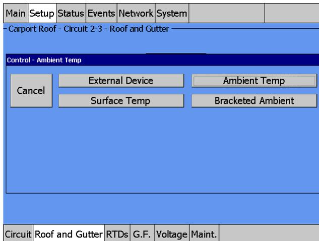
Fig. 3.84 Roof & Gutter - Bracketed Ambient Temperature Control Window
