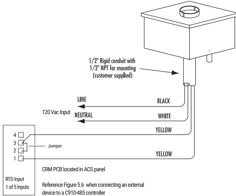
Fig. 5.9 Connecting the LCD-7
