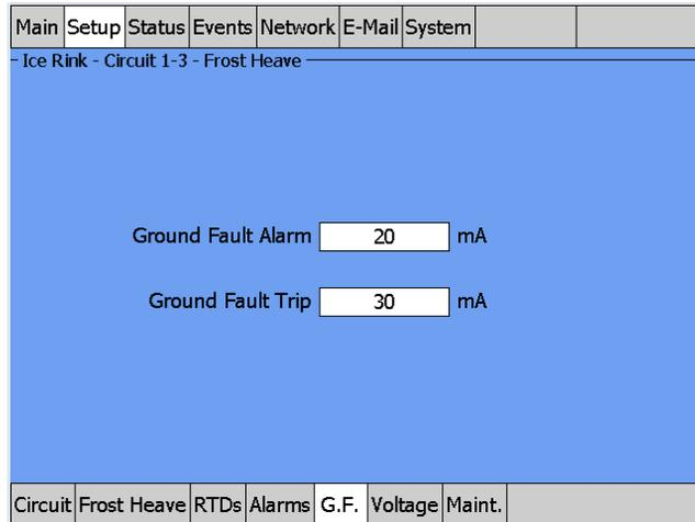
Fig. 3.15 Setup|G.F. window (Frost Heave)
