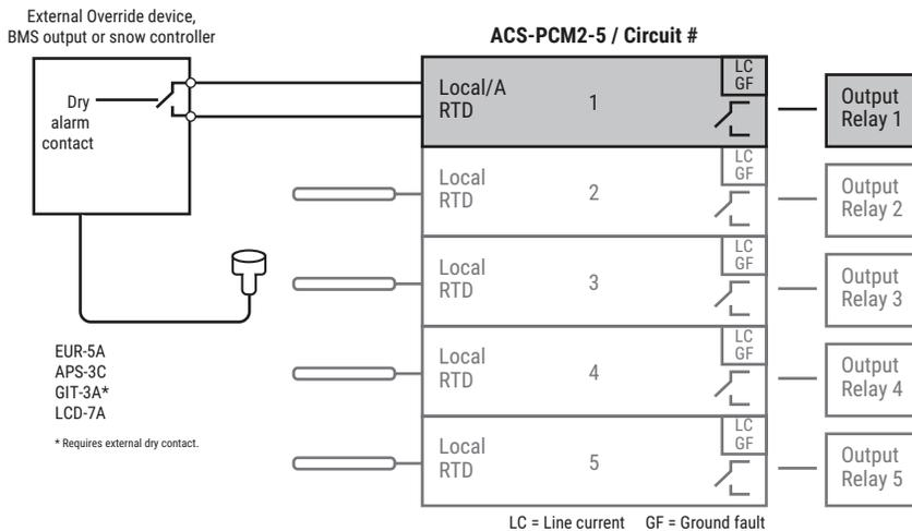
Fig. 5.5 External Device Control
