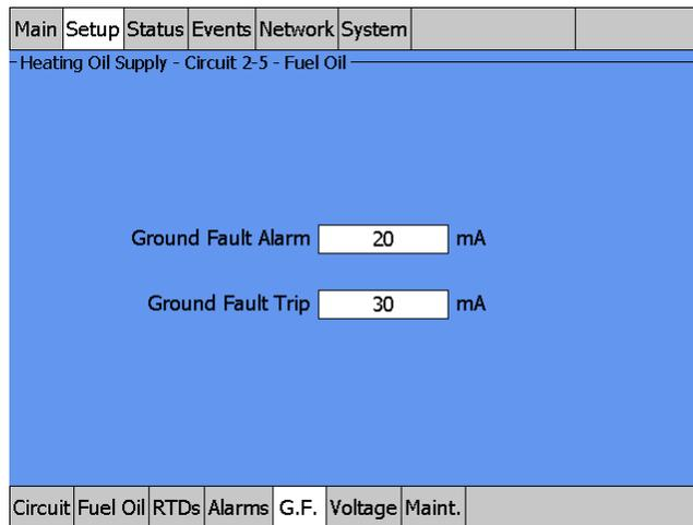
Fig. 3.56 Setup|G.F. window (Fuel Oil Line Control)
