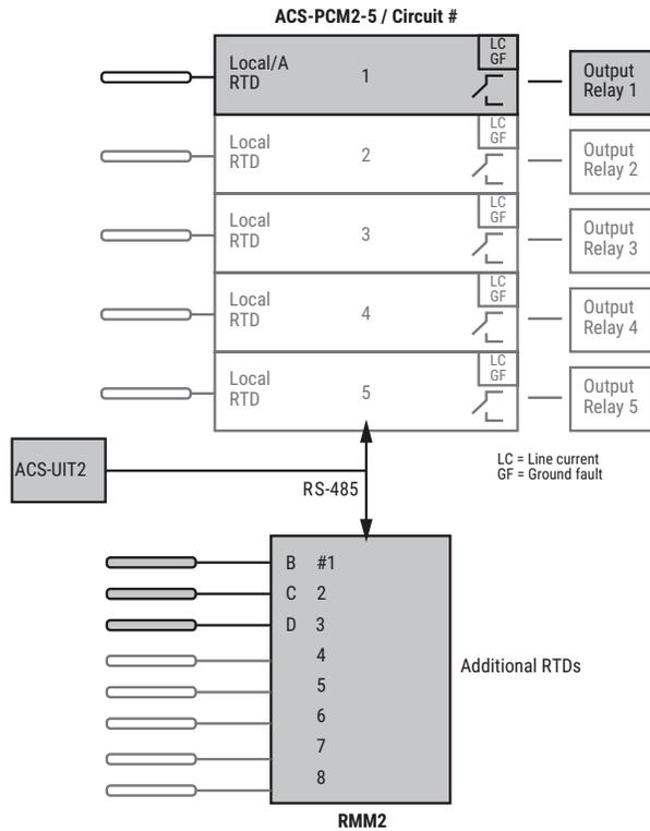
Fig. 1.4 Multiple RTD input control circuit
