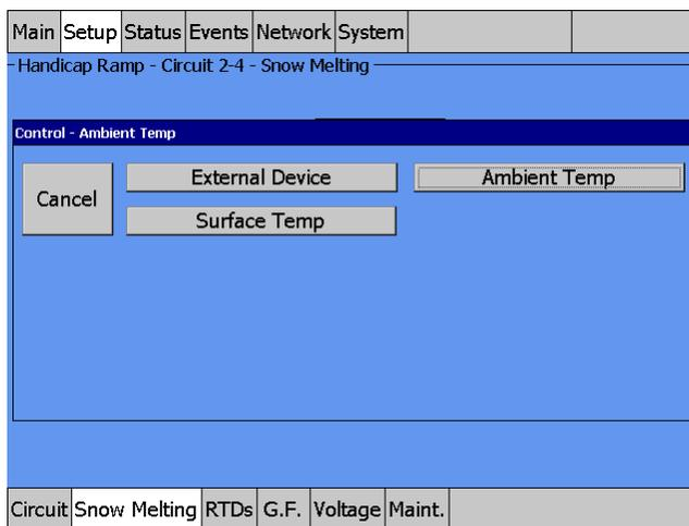
Fig. 3.96 Snow Melting External Device Control window
