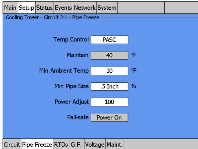
Fig. 3.39 Setup|Pipe Freeze PASC Control window
