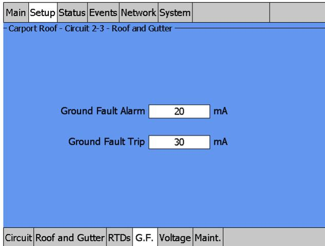
Fig. 3.87 Setup|G.F. Window (Roof & Gutter - Bracketed Ambient Temp Control)
