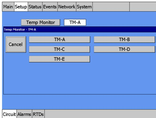
Fig. 4.2 Temp Monitor - Assign Circuit Window
