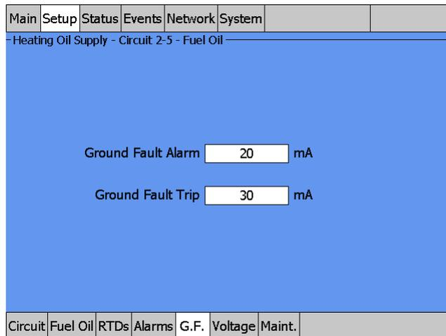
Fig. 3.63 Setup|G.F. window (Fuel Oil PASC Control)
