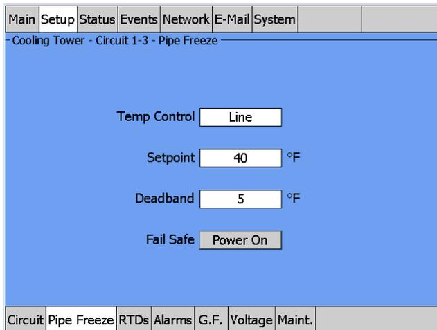
Fig. 3.32 Setup|Pipe Freeze Line Control window
