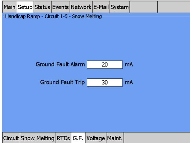
Fig. 3.99 Setup|G.F. Window (Snow Melting External Control)
