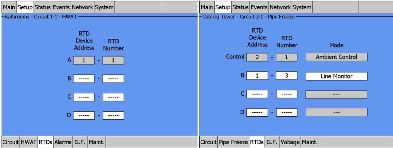
Fig. 2.18 Assigning additional RTDs.
