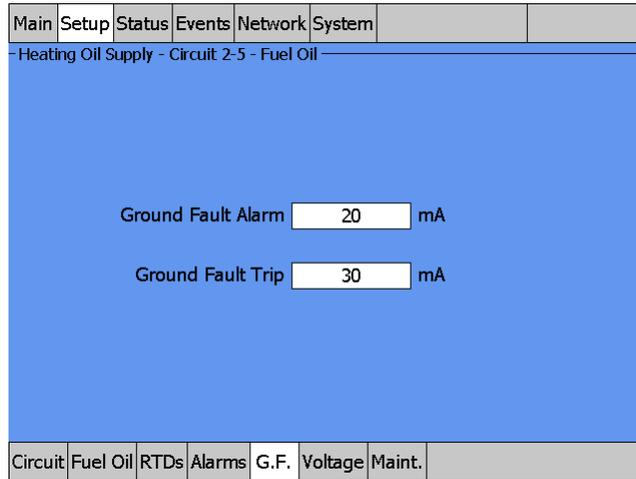
Fig. 3.49 Setup|G.F. window (Fuel Oil Ambient Control)
