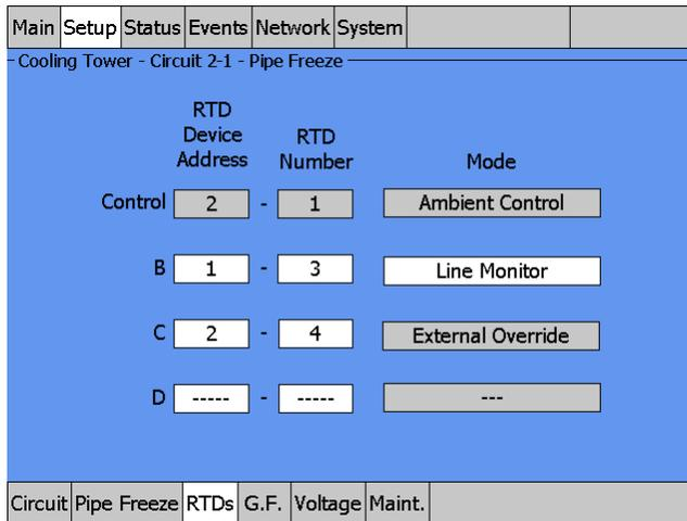
Fig. 3.40 Setup|RTDs window (Pipe Freeze PASC Control)
