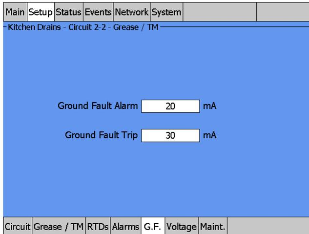
Fig. 3.69 Setup|G.F. window (Grease/TM Waste)
