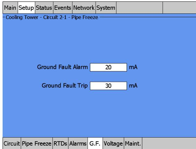
Fig. 3.35 Setup|G.F. window (Pipe Freeze Line Control)
