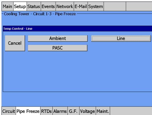
Fig. 3.31 Pipe Freeze Temperature Line Control window
