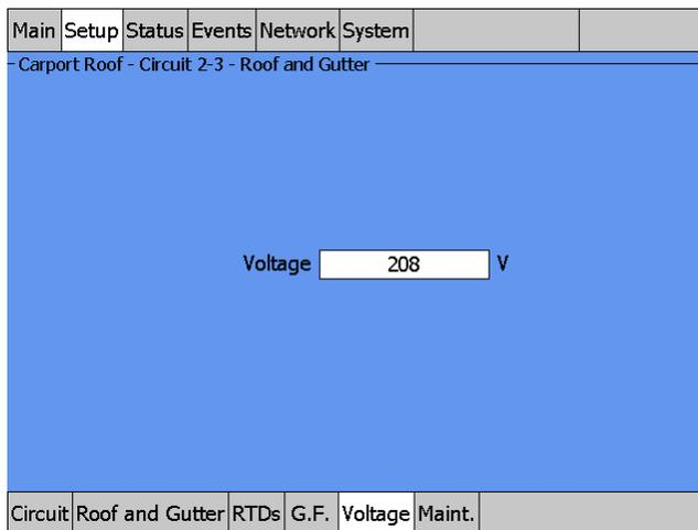
Fig. 3.88 Setup|Voltage Window (Roof & Gutter - Bracketed Ambient Temp Control)
