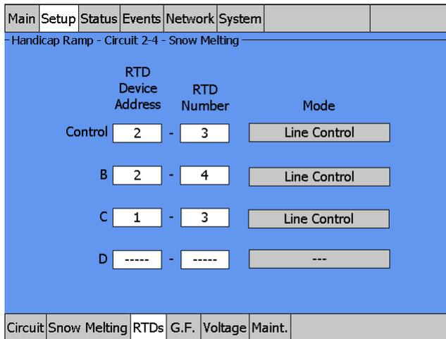
Fig. 3.110 Setup|RTDs Window (Snow Melting Surface Temp Control)
