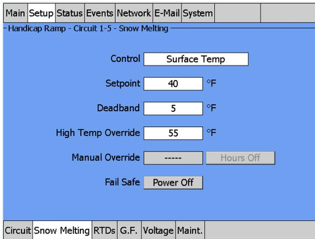
Fig. 3.109 Setup|Snow Melting - Surface Temp Control Window
