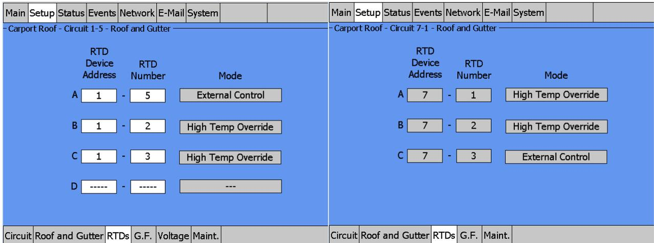
Fig. 3.74 Setup|RTDs window (Roof & Gutter External Control)
