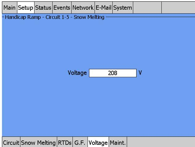
Fig. 3.100 Setup|Voltage Window (Snow Melting External Control)
