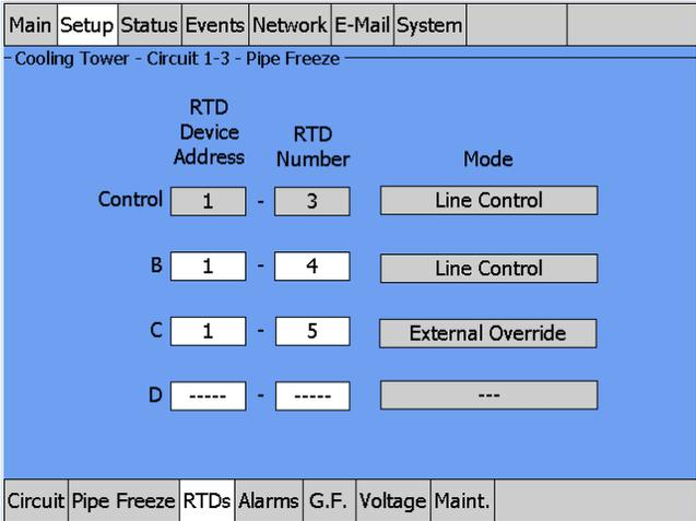
Fig. 3.33 Setup|RTDs window (Pipe Freeze Line Control)
