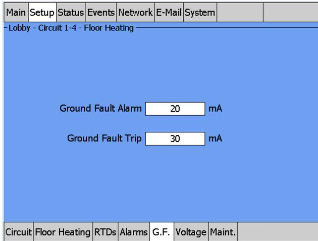
Fig. 3.21 Setup|G.F. window (Floor Heating)
