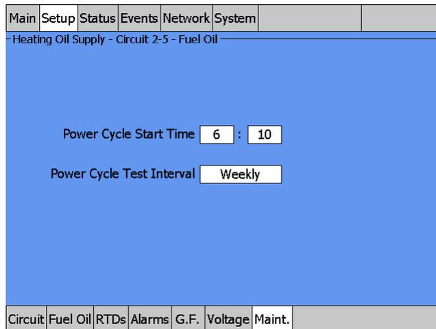
Fig. 3.65 Setup|Maint. window (Fuel Oil PASC Control)
