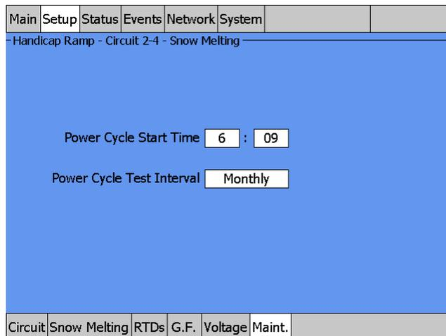
Fig. 3.95 Setup|Maint. Window (Roof & Gutter - Surface Temp Control)
