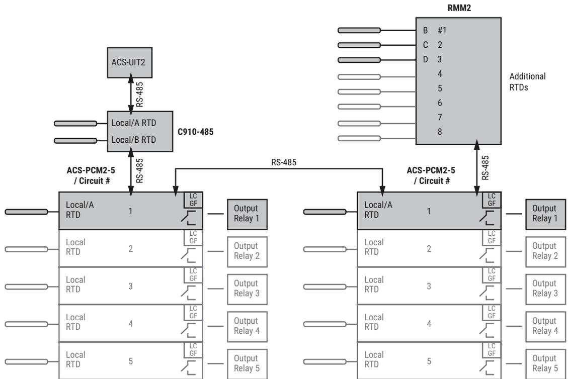
Fig. 1.5 Multiple ACS-PCMs, C910-485 and RMM2
