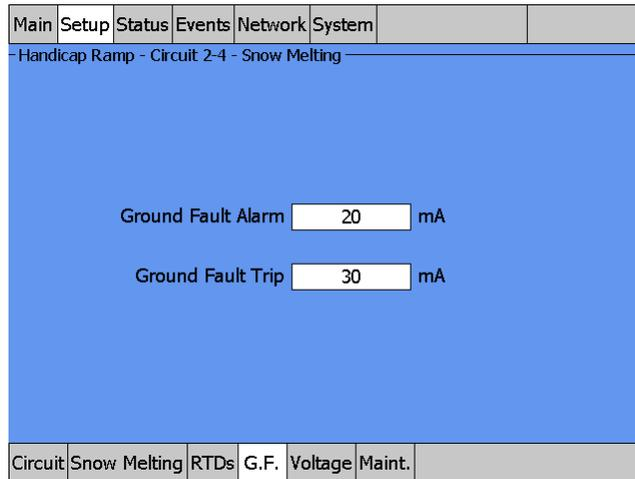
Fig. 3.105 Setup|G.F. window (Snow Melting Ambient Control)
