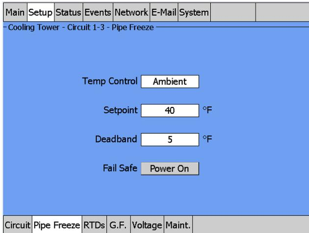
Fig. 3.25 Setup|Pipe Freeze Ambient Control window
