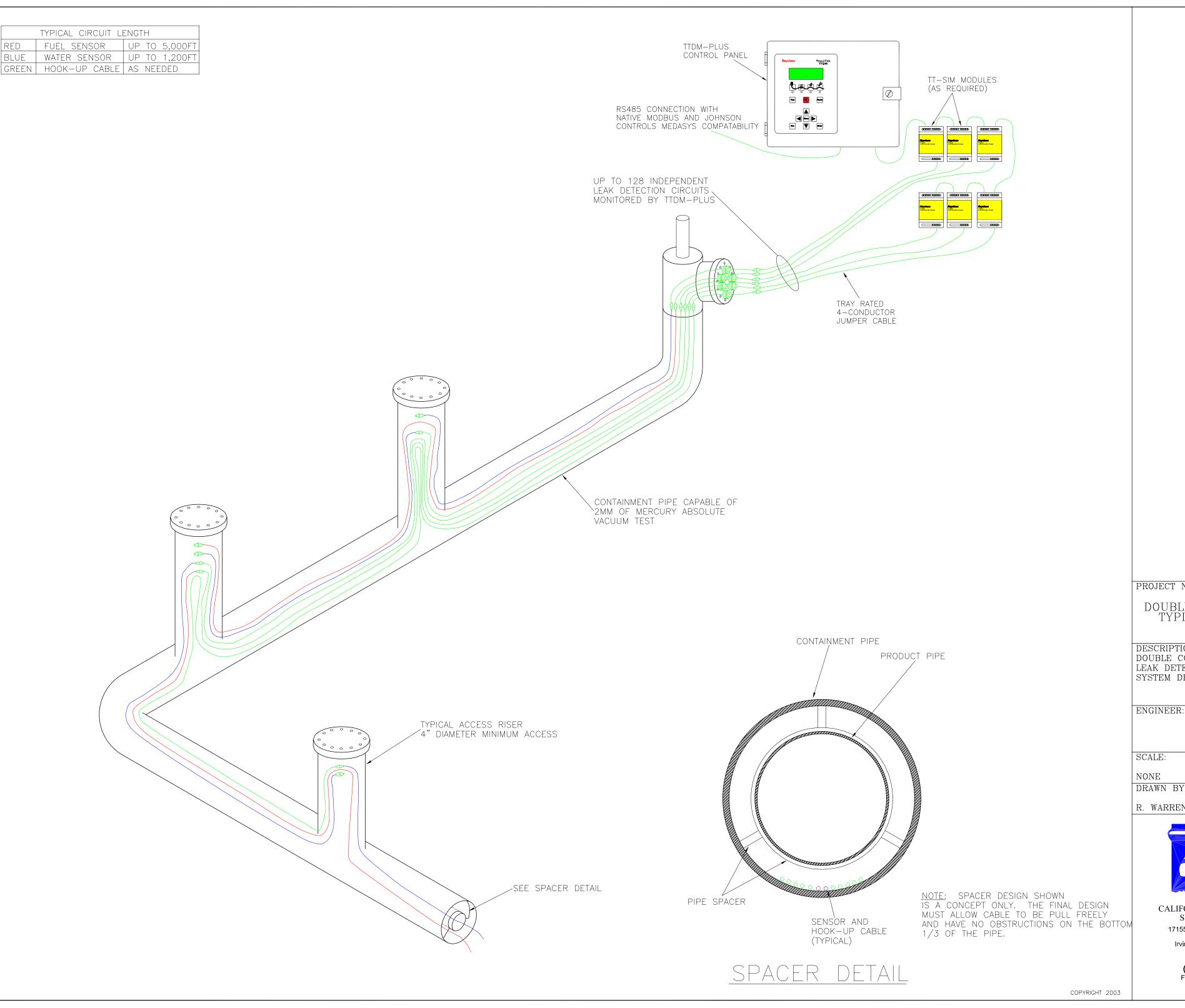
PROJECT NAME: PIPELINE DOUBLE CONTAINMENT TYPICAL DRAWING
